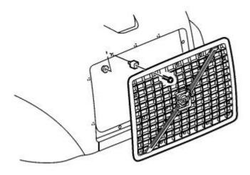
Install the grille using the fasteners previously removed. Torque fasteners to 2 Nm (1.5 in-lb).
