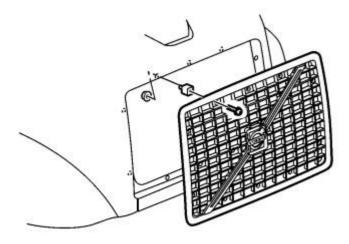
Remove fasteners securing the grille to the vehicle and remove the grille. Place the grille out of the work area.
