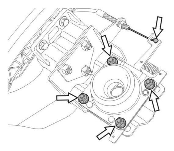
Remove the four hood latch mounting bolts. Remove the hood latch.
